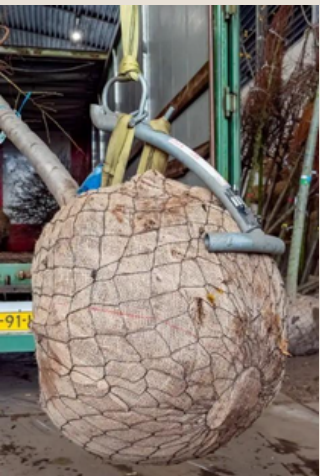
Fig. 2: Tree Handling with a rootball hook
